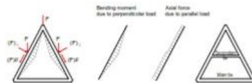
Figure 5: Effect of non-apex loading.
